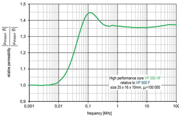
Fig. 15: Relative permeability between VITROPERM 550 HF and VITROPERM 500 F for cores of the size of 26 x 16 x 10 mm.
