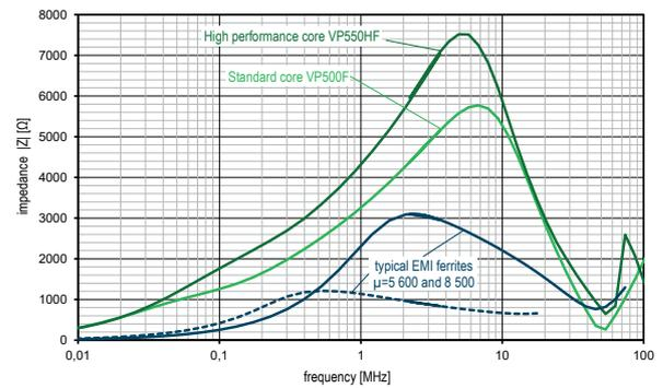
Fig. 16: Comparison of the impedance  $|Z| (f)$  of VITROPERM 550 HF vs. VITROPERM 500 F and typical ferrites. In each case, the core size is 25 x 20 x 10 mm, wound with 14 turns.
