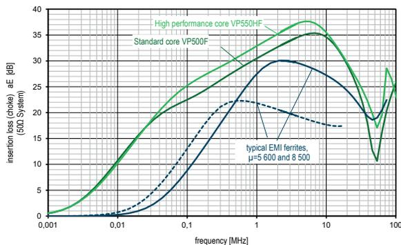
Fig. 17: Comparison of the insertion loss  $aE (f)$  of VITROPERM 550 HF vs. VITROPERM 500 F and typical ferrites. In each case, the core size is 25 x 20 x 10 mm, wound with 14 turns.
