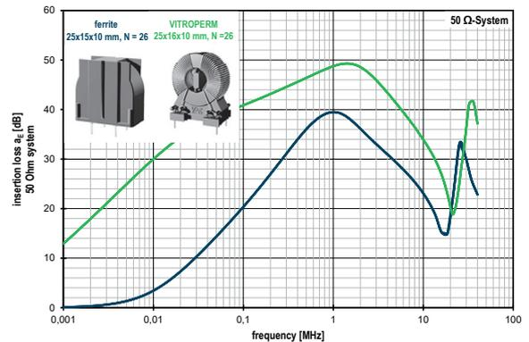
Fig. 13: Comparison of insertion loss curve of a VITROPERM 500 F CMC (green curve) and ferrite CMC (blue curve) of similar size and with the same number of turns
