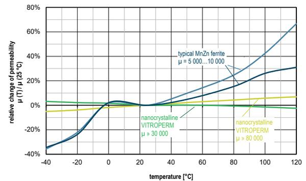
Fig. 10: Relative change of  $\mu(T)$  at  $f = 100$  kHz, normalized for room temperature
