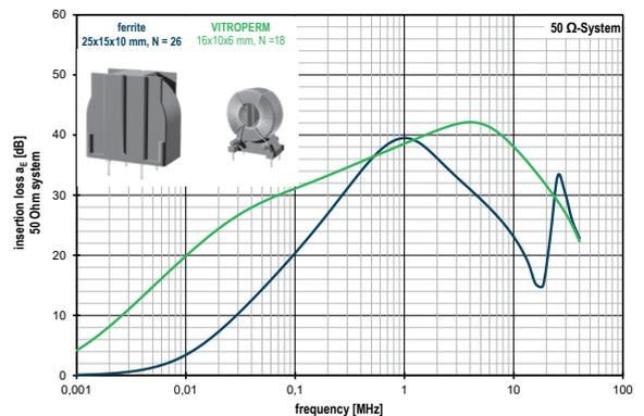
Fig. 14: Comparison of the dimensions of a VITROPERM 500 F CMC (green curve) and ferrite CMC (blue curve) with similar attenuation properties in the 1 MHz range
