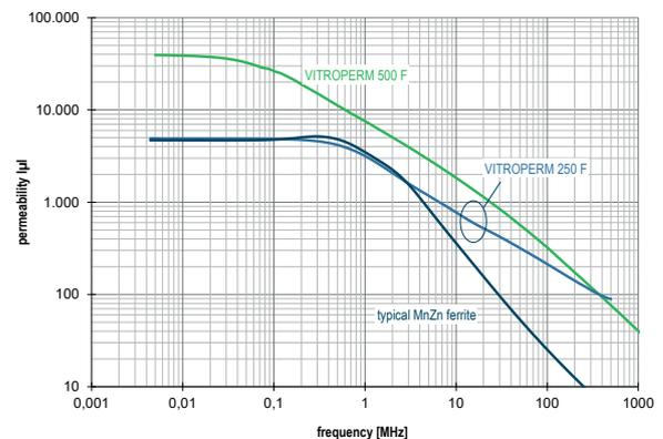
Fig. 6: Frequency response of the permeability of VITROPERM 500 F ( $\mu = 40,000$ ) and VITROPERM 250 F ( $\mu = 5,000$ ) in comparison to a typical MnZn ferrite ( $\mu = 5,000$ )
